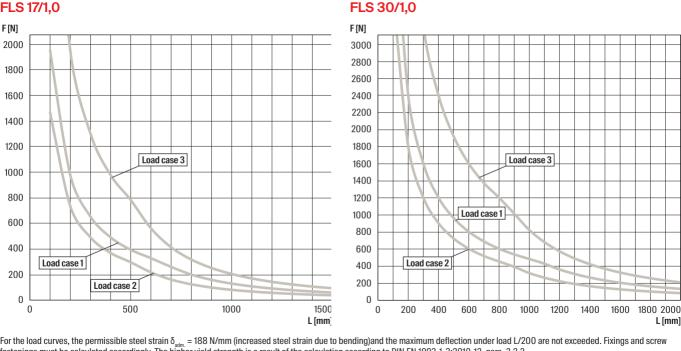
fastenings must be calculated accordingly. The higher yield strength is a result of the calculation according to DIN EN 1993-1-3:2010-12, para. 3.2.2.
