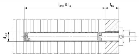
The fischer filling disc FFD can be used instead of a washer in all installation conditions and allows the annular gap to be subsequently injected with adhesive.
