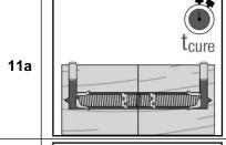
After the period of time until the adhesive has reached its final joint strength at T  $\leq$  60 °C (t<sub>cure</sub>) in accordance with **Table B7.2**, the assembled structural component may be fully loaded.
