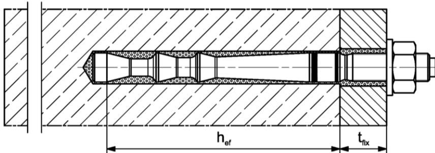
**Pre-positioned or push through installation with subsequently pressed filling disk**
